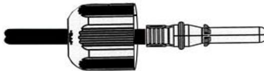
Figure4-13 Crimp the negative metal terminal
