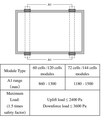
Method B: Use four clamps on the short side. Mounting rails run parallel to the long side frame.
