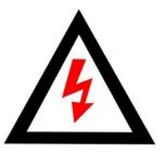
30 Volts or higher is potentially lethal. Please use insulated tools and rubber gloves when working with modules in sunlight.
