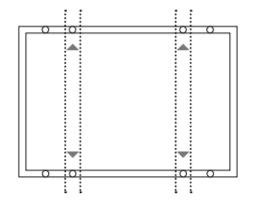
The long side frame is installed with 4 bolt mounting holes on the outside or inside. Mounting rails run perpendicularly to the long side frame.
