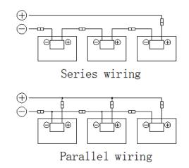
An appropriately rated over-current protection device must be used when the reverse current could exceed the value of the maximum fuse rating of the modules. An over-current protection device is required for each series string if more than two series strings are connected in parallel.
